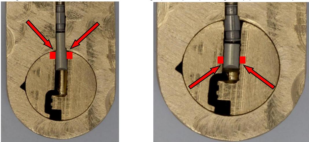
**Picture 35a and 35b: A high lifted pin and a short pin.**
