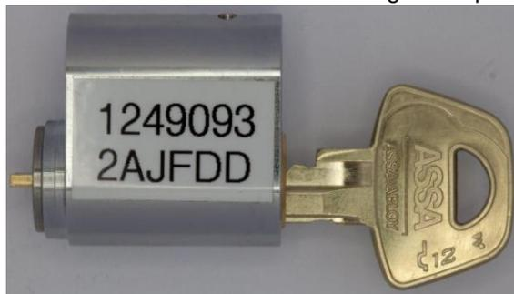
**Picture 20: The level 1 key does not go all the way into a level 2 cylinder**
