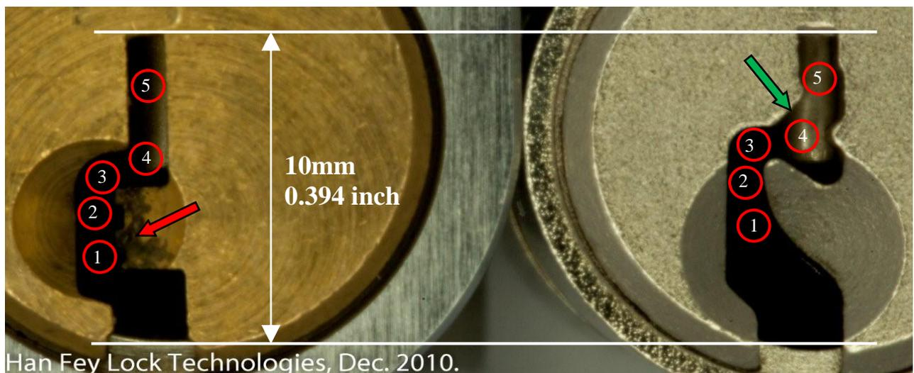
**Picture 54: Detailed picture of ASSA d12 keyway and Abus TS5000 keyway**
