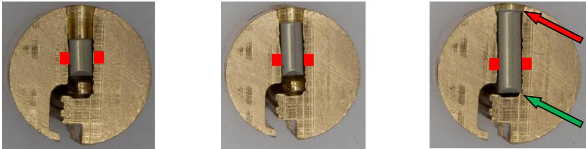
**Picture 36a, 36b and 36c: Different “shielding” positions of the bottom pins**
