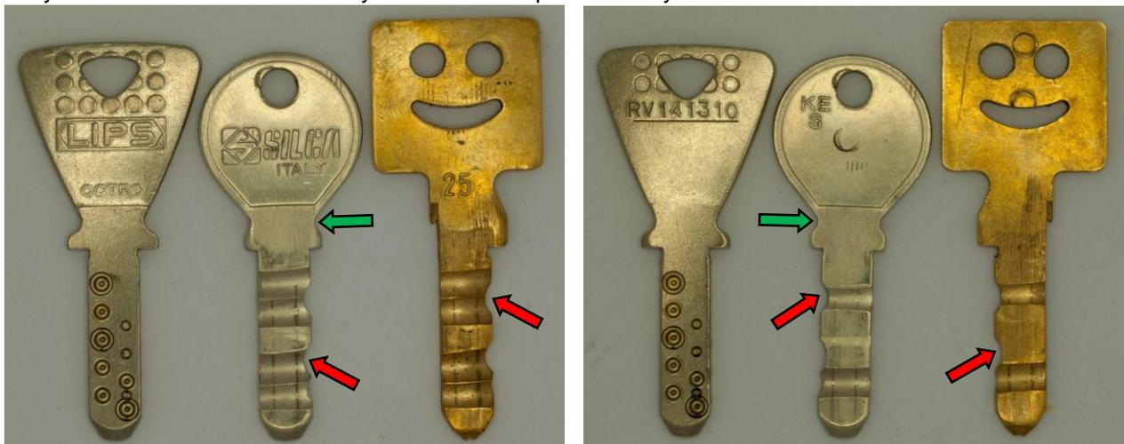
**Picture 56a and 56b: Left and right side of the impressed Lips Keso keys**
