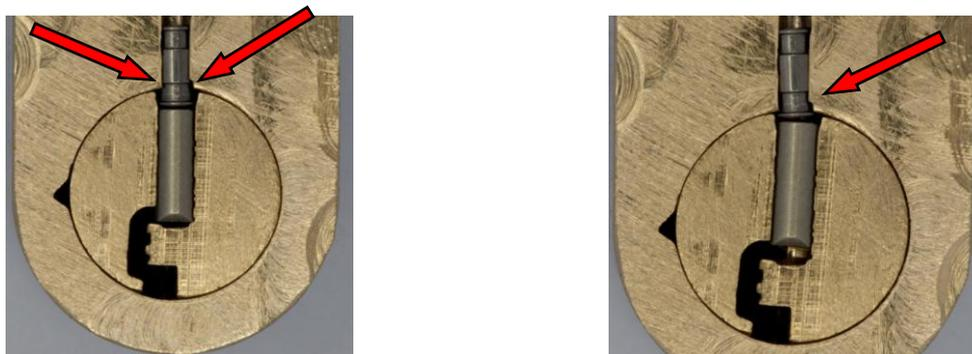
**Picture 37a and 37b: Plug in locked position and tilting top pin in the housing**
