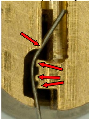
**Picture 42: Detail of the keyway with the "anti-slip" ribs and the 0.45mm wire.**
