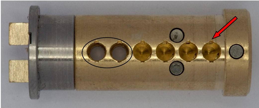
**Picture 25: The plug without pins**
